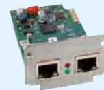
LRZ 923 EtherCAT module with RJ45 connection
