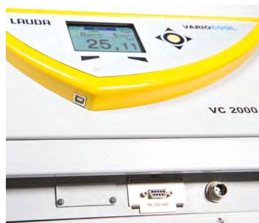
Standard-issue USB interface and alarm contact as well as additional optional interfaces that can be retrofitted
