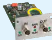
LRZ 922 EtherCAT module with M8 connection
