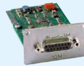
LRZ 915 Contact module with 3 inputs and 3 outputs
