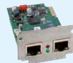
LRZ 923 EtherCAT module with RJ45 connection
